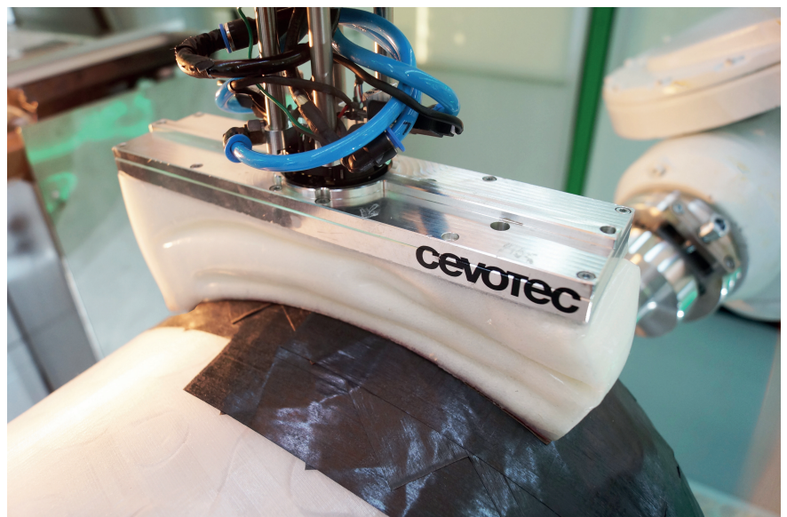
Fig. 4. The robotic system places the reinforcement patches directly on the dome areas of the pressure vessel. © Cevotec
